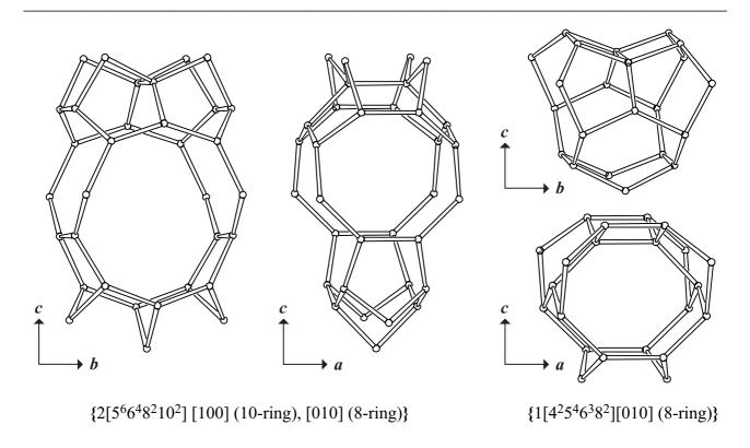
Figure 4. Channel intersection viewed along a (left), and along b (middle) and interconnecting cavity between 10-ring channels (right) viewed along a (top), and along b (bottom).
