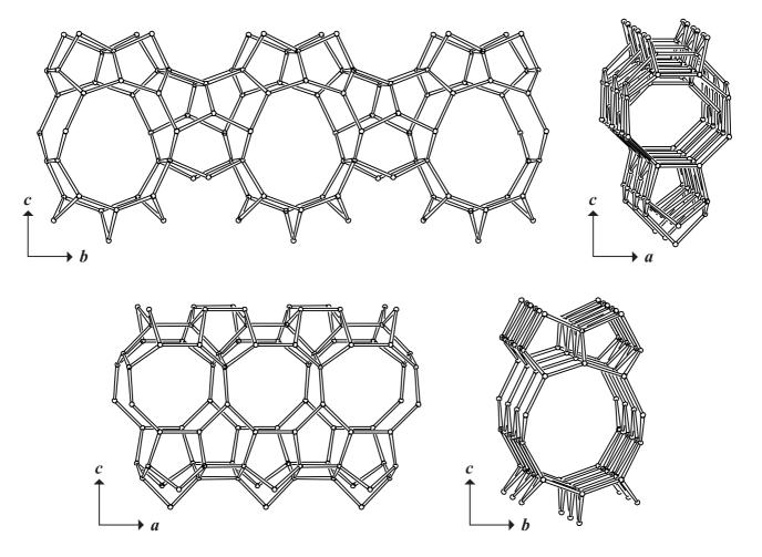
Figure 5. 10-Ring channels, parallel to a, are interconnected along b through cavities composed of fused 5- and 6-rings that are part of the wall of an 8-ring channel parallel to b (top). View along a (left), and along b (right); fusion of channel intersections along a (bottom), viewed along b (left) and along a (right).
