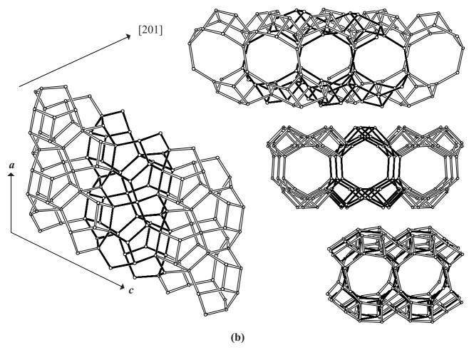
Figure 5 [Cont'd]. (b): Fused channel intersections in **RRO** viewed along b (left) and (from top right to bottom right) along [201], a and c.
