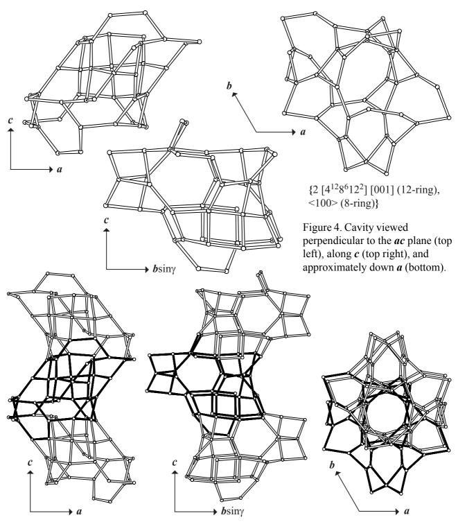
Figure 5. Fusion of cavities into a chiral channel of strongly distorted 12-rings and 8-rings along *c*.
