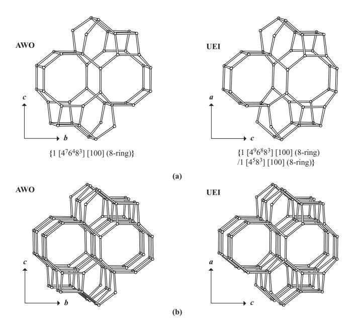
Figure 4. (a): Large cavities in **AWO** seen along a (left) and in **UEI** along b (right); (b): Interconnected channels parallel to a and b are formed when cavities in **AWO** and **UEI** are linked along a (left) and along b (right), respectively.
