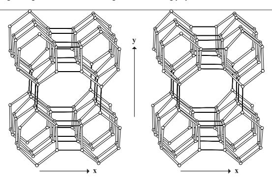
Figure 2. Connection mode (1) in AWO (left) and connection mode (2) in UEI (right) seen along z.
