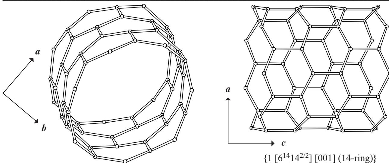
Figure 3. Channel with 14-ring window in **DON** viewed along  $c$  (left), and along  $b$  (right). ▲
