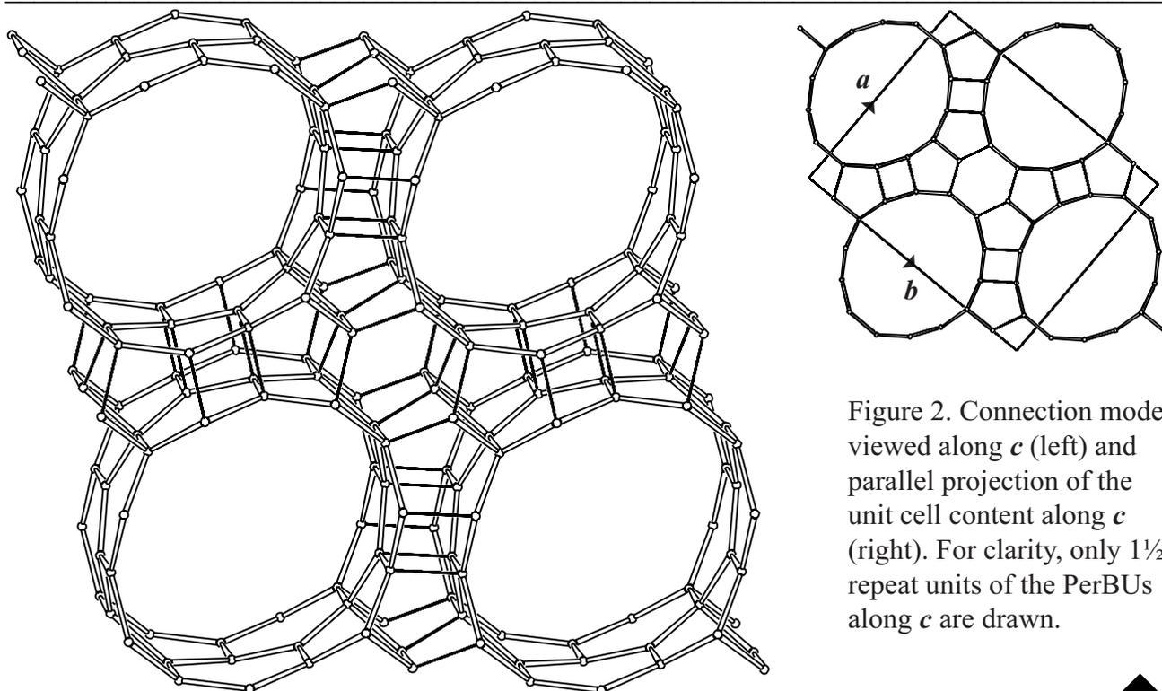
Figure 2. Connection mode viewed along  $c$  (left) and parallel projection of the unit cell content along  $c$  (right). For clarity, only  $1\frac{1}{2}$  repeat units of the PerBUs along  $c$  are drawn.
